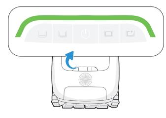
3 Place the robot on a level surface and wait for about 5s for it to calibrate
