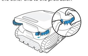
2 Install it onto the robot with the interface facing down
